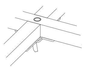
2 SCREW IN WING-NUT AFTER UNFOLDING
