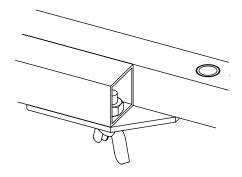
1 UNSCREW WING-NUT & UNFOLD
